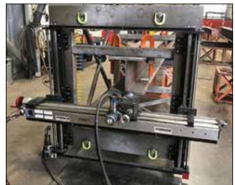
I-Beam end face milling with a GMRF1000. ►
