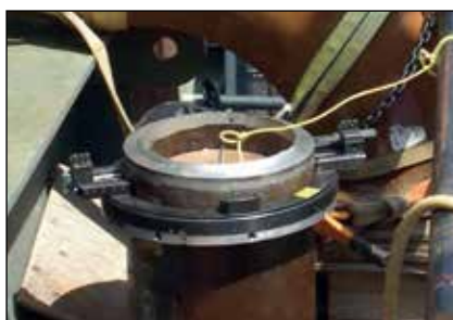
◀ NB-model narrow body clamshell cutter.
