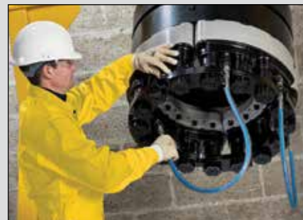
▲ Multi-Stud Tensioning application.
