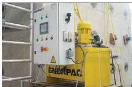
◀ Custom pumps with control packages.
