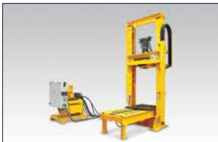
◀ 100-Ton Press for Assembly of Spring-Loaded Cylinders
