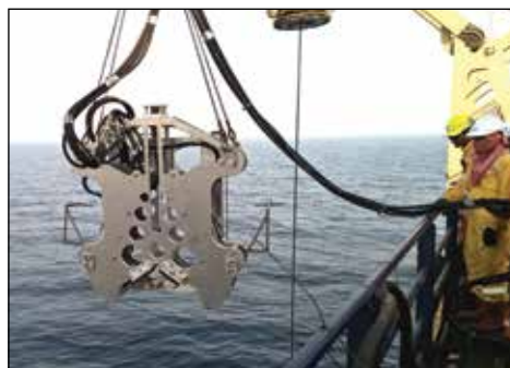
▲ MDWS Diamond Wire Saw lowered into sea.
