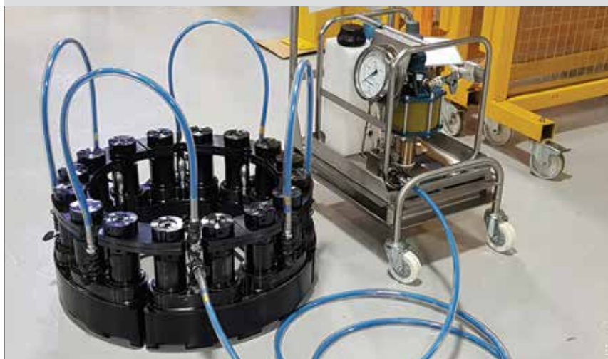
▲ Multi Stud Tensioning Set-Up.
