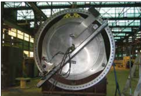
▼ Wind tower machining with WP4600.
