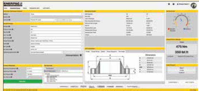
▲ Standard flange calculation menu (INFORMATE)
